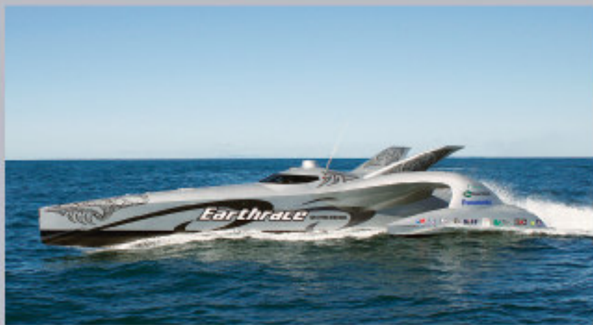
Above: Earthrace is a B100-powered 78-foot trimaran with carbon fiber and Kevlar laminates and engine air intakes atop her "wings" to facilitate breathing in the wave-piercing mode. Below: Earthrace 's proposed around-the-world route.
